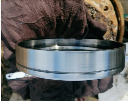
Seal bushing - TEKAD 1000 coating - DED process
