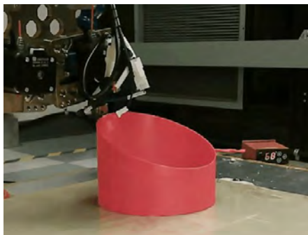
Figure 3 – 3D printing of a truncated cylinder with a 2:1 front to back ratio with constant number of layers from PLA by FFF method.
