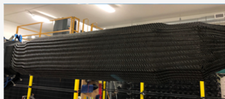
Figure 1 – 3D printed ABS mandrel covered by a carbon fibre braid.
