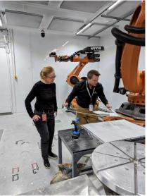
At PolyCSAM, many different metals were deposited as samples to create a colour pallet for the artist to work with. It was decided that we would be using 6 metal powders, each with a distinct shade of grey. The thickness of each layer, determined by the artist, could be controlled by the velocity of the spray gun. Shims were adhered to the back of the masks and adjusted between sprays to ensure a consistent standoff between the mask and the substrate, as
