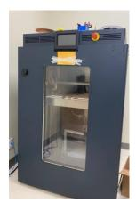
**Purpose:** Printing large high-performance thermoplastics in a heated chamber.
