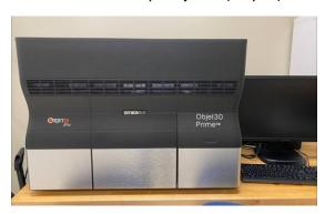
**Purpose:** A thermoset 3D printer based on the Polyjet technique that prints high-resolution and versatile prototypes for a variety of applications.
