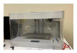
**Purpose:** Printing thermoplastic polymer-based composite parts reinforced with continuous glass or carbon fibers.
