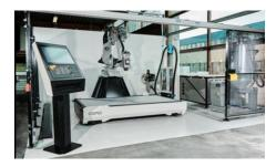
Purpose: A large-scale thermoplastic composite 3D printer integrated with CNC milling equipment
