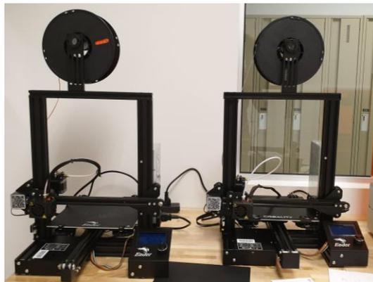
**Purpose:** Printing thermoplastics for prototyping, experimenting, learning, etc.
