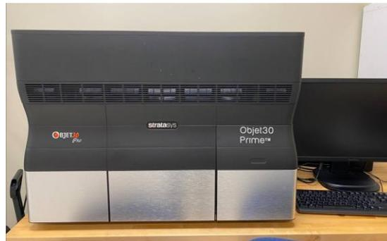
**Purpose:** A thermoset 3D printer based on the Polyjet technique that prints high-resolution and versatile prototypes for a variety of applications.
